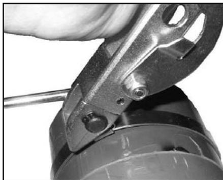
**8.** This stub should be shortened. With cutter in the open position, Place tool over stub, insert into slot and trim off excess.
