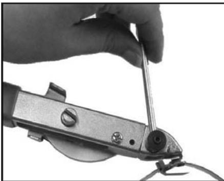
**4.** Cut off excess band by lifting cutter lever.
