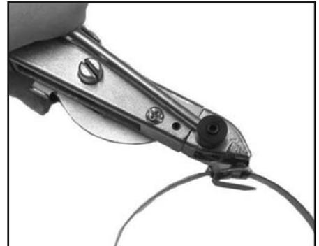
**3.** When sufficient tension has been applied, release locking pawl and rotate tool over object being clamped. Note: For extra strength double-wrapped band is recommended.
