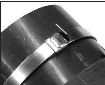
**7.** Insert tail of the preformed clamp into the tool. Tension as shown in steps 2 & 3. When tensioned sufficiently, release locking pawl and rotate over object being clamped. Cut off, leaving stub.
