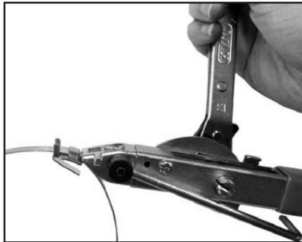
**2.** Form a clamp by threading the band through buckle and make a fold under the buckle. Insert tail of clamp into head of tool and slide into slot of winding mandrel. Depress locking pawl and tension clamp with forward strokes of the ratchet wrench.
