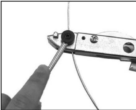
**1.** Cut off adequate band from roll of 1/4" or 3/8" band by opening the slot in the head of the tool with the cut off lever at right angles to the tool. Thread the band through the slot and cut.
