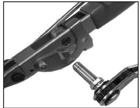
**6.** Remove band wrapped around winding mandrel by lifting up on locking pawl. Reverse ratchet and withdraw tensioning wrench from tool.
